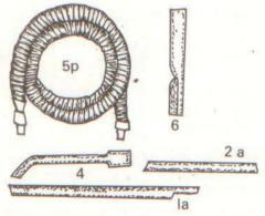
la - Suction tube, Im 2a - Suction tube, 0.5m 4 - Suction nozzle 5p - flexible hose for suction (5m) 6 - flat nozzle Special accessories at extra cost
